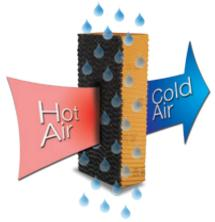
The larger the amount of water evaporated from air, the higher the temperature reduction shall be. Also, the dryer the air or the lower the relative humidity, the greater the possibility of evaporation will be.
